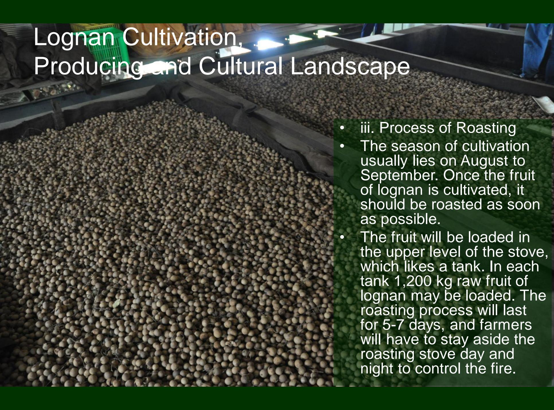
A large industrial roasting stove filled with lognan fruit. The stove is a long, rectangular metal tank divided into sections. The fruit is piled high in the sections. In the background, there are some lights and a person's legs in blue jeans.
