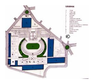
FIG 2 Original 1960s site plan showing the important moats for drainage and water treatment station that are an integral part of the design
