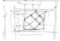
FIG 11 architect's sketch showing the unusual concept of a square within a square and its relation to the site in which the 45° angle offers good aspects to all four sides
