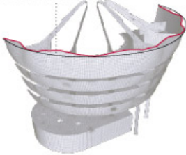
Exaggerated view of wall movement
