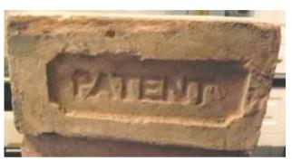
This wire cut brick was produced by the Hobart Town Patent Brickwork. A Clayton's double action machine and pressed brick machine were in use at the Hobart Town Patent Brickworks in New Town which was up for sale in 1857. (Photos courtesy of K. Bone)
