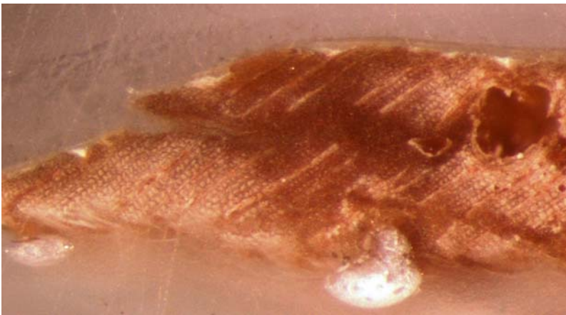
Figure 2. Limed finish of an internal door in the rear (children's wing), as seen in a cross-section under a reflected light microscope (63x). The large brown area is timber, with small amounts of white paint visible in indentations on the surface, beneath a layer of transparent varnish. (N Schmeder, 2014)
