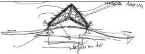
FIG 15 architect's sketch showing the climatic response of the double-layered roof and cross ventilation
